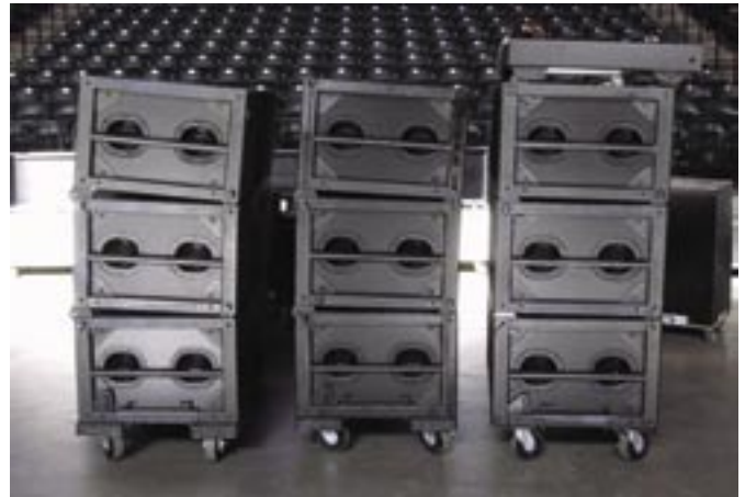
Figure 33. M3D blocks ready for transport with vertical splay left in
